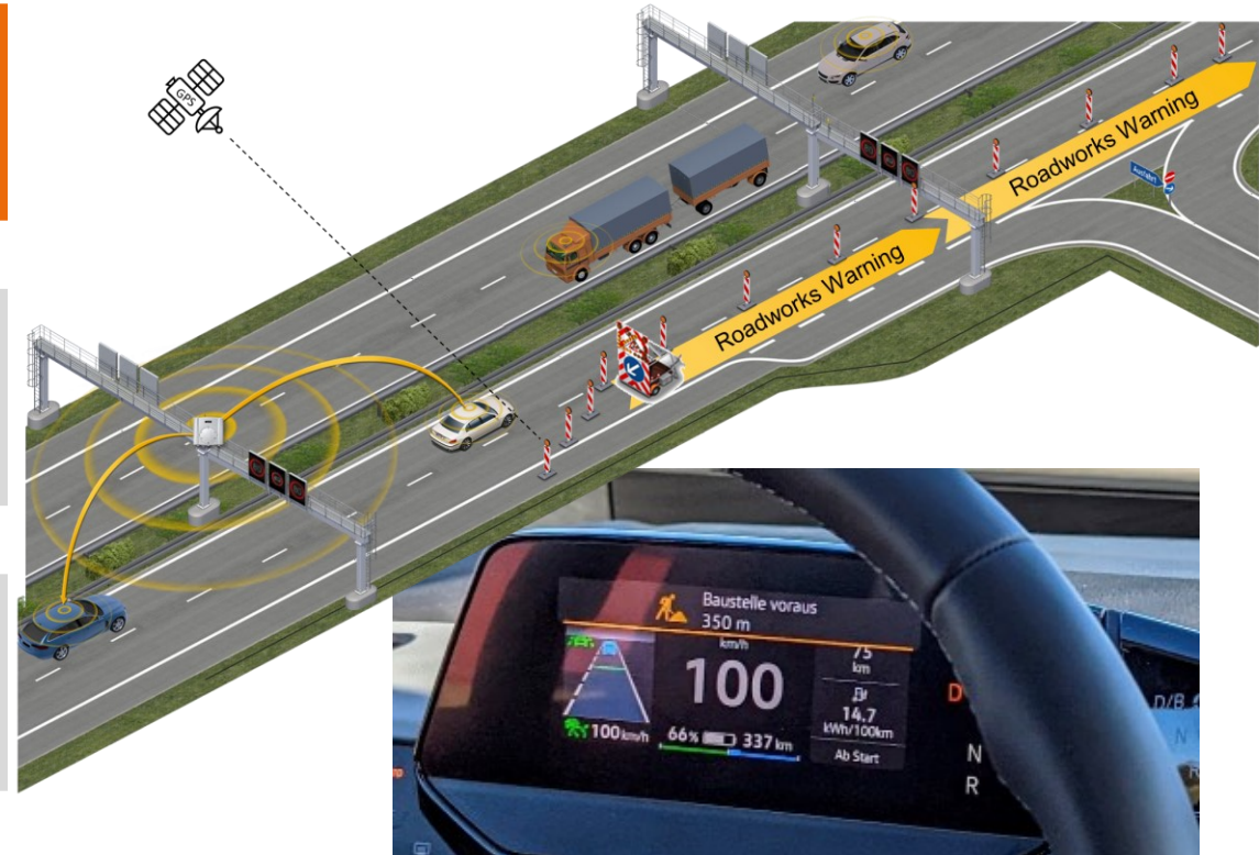
C-ITS Roadworks Warning in VW ID.3
