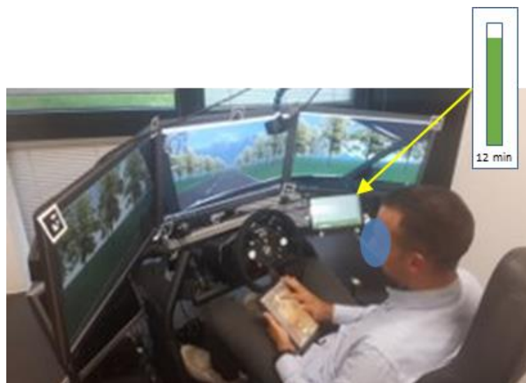
Figure 1 Experimental Set-up to Evaluate the Benefits of Displaying the Driver the Duration of the Automated Drive
