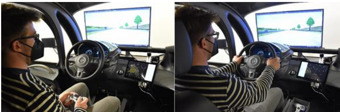
Figure 6: (left) seating position for automated driving; (right) seating position for manual driving
