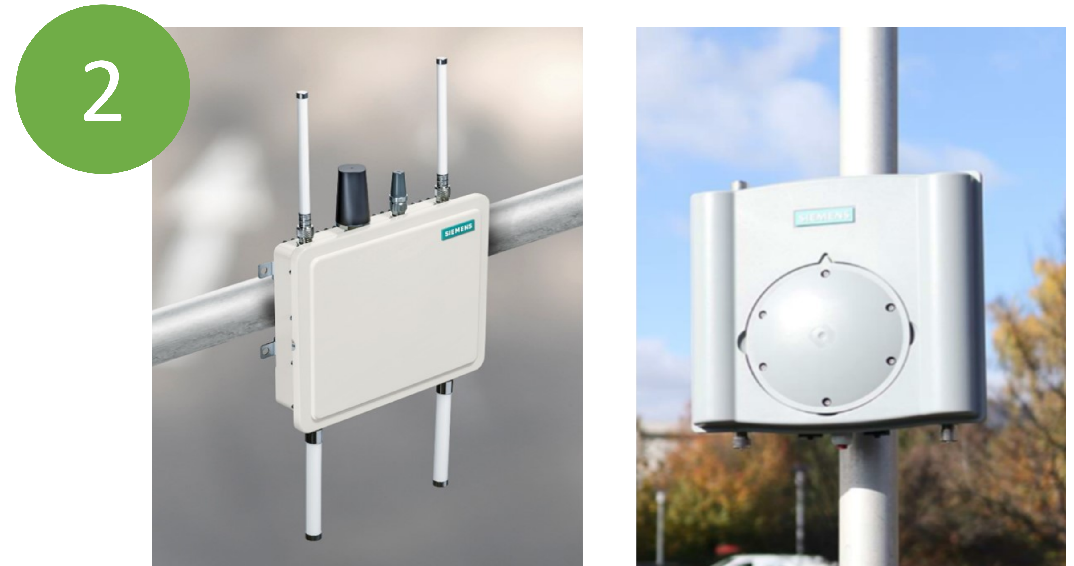
The obstruction information is communicated via road-side unit to the vehicle using standardized C-ITS messages (IVIM, DENM) etc.
